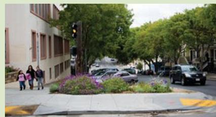
**Bulb Outs with Green Infrastructure:** A traffic calming method that extends the sidewalk, reducing the distance to cross the street increasing pedestrian visibility and safety. These may include various green technologies to capture and treat stormwater.
