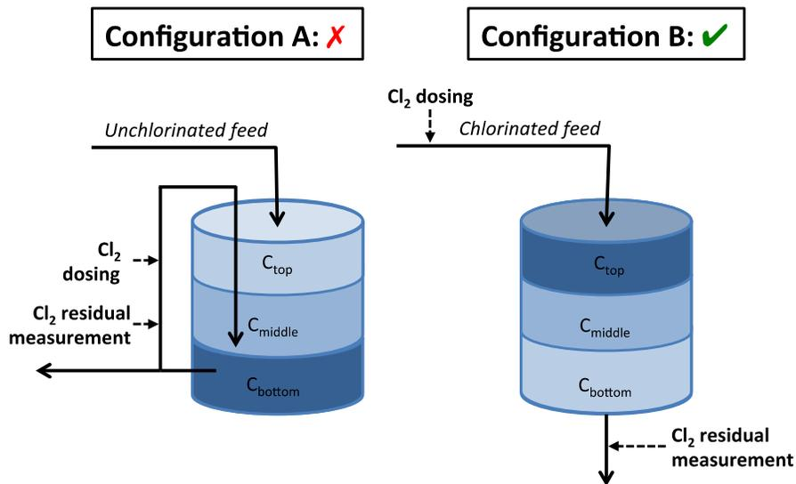
A Continuous Stirred Tank Reactor (CSTR) is the least ideal configuration for a chlorine contact basin, but can use a baffling factor of 0.1. In a CSTR, some volume of water leaves immediately upon entering the basin and thus experiences zero contact time. The more plug flow-like your chlorine basin, the less likely that water will be discharged from the basin with little to no contact time.
