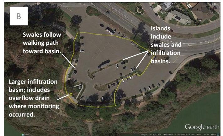
Figure 2. (A) Flows at Sunset Circle were simulated for the pre-construction conditions using SWMM hydrologic modeling software. (B) Post-construction flows were measured in a catchbasin (at yellow circle) located within the large infiltration basin in the southwestern point of the parking lot. Catchment boundary in both aerials shown as yellow outline.
