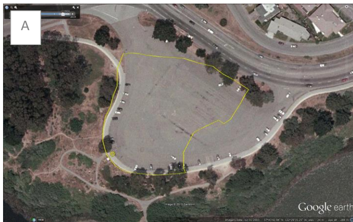
Figure 2. (A) Flows at Sunset Circle were simulated for the pre-construction conditions using SWMM hydrologic modeling software. (B) Post-construction flows were measured in a catchbasin (at yellow circle) located within the large infiltration basin in the southwestern point of the parking lot. Catchment boundary in both aerials shown as yellow outline.
