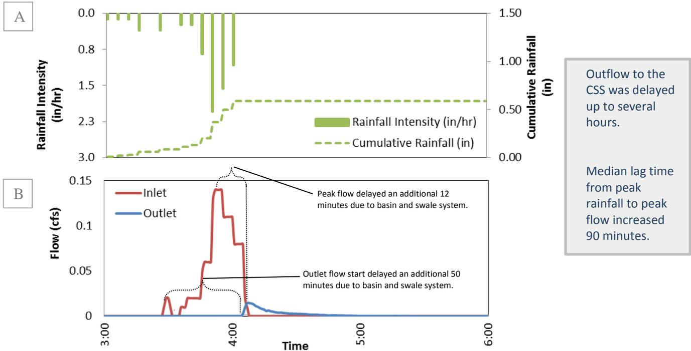
Figure 5. A) Rainfall intensity and cumulative rainfall during a storm event on April 12, 2012. B) Storm hydrograph showing inlet and outlet flow rates and annotated lag times during this storm event.
